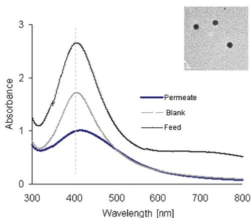
Fig. 1. UV–vis absorbance spectra of Ag-NPs in feed and permeate of UF through 0.01  $\mu\text{m}$  PC membrane. The inset is a representative transmission electron microscopy (TEM) micrograph showing the shape and size of a few particles (bar = 20 nm).
