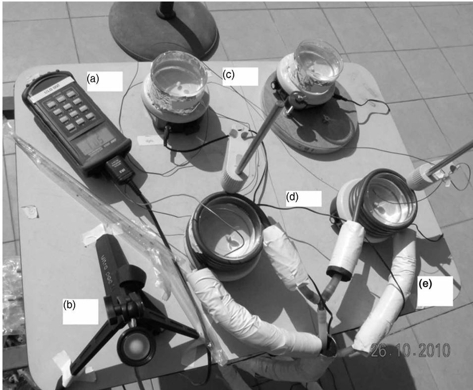
Figure 1 | Field experiment set-up: (a) thermocouple, (b) spectroradiometric detector, (c) glass dishes exposed to solar radiation only, (d) test dishes exposed to solar radiation and heat via water flowing through the copper tube, (e) insulation layer around the silicone tube that connects the copper tube to the cooler.
