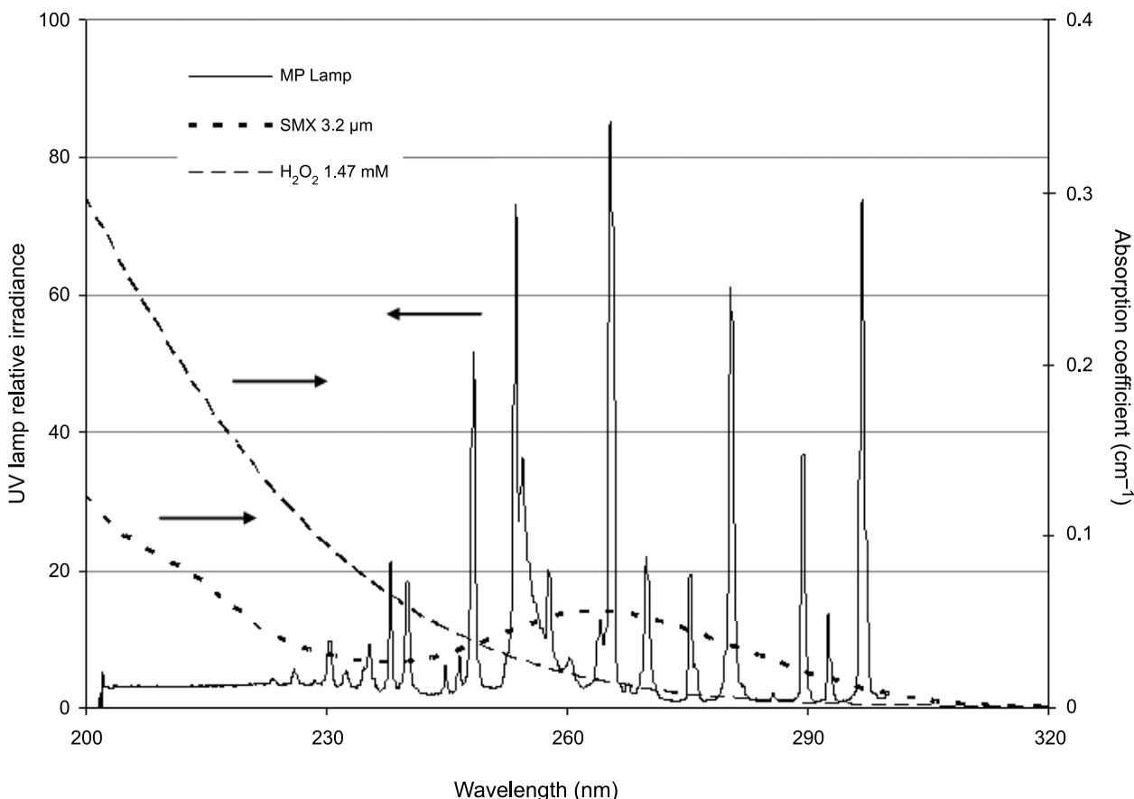
Figure 2. Emission spectra of the UV lamp and absorption spectrum of SMX (3.2  $\mu\text{M}$ ) and  $\text{H}_2\text{O}_2$  (1.47 mM) in DI water (pH 6.0).
