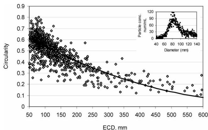
**Figure 5.** Circularity versus ECD for latex bead particles. The insert represent the PSD of the latex beads.
