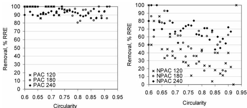
**Figure 3.** Percent removal of particles as function of circularity for PAC (left image) and NPAC (right image) samples after 120, 180, and 240 min of filtration.
