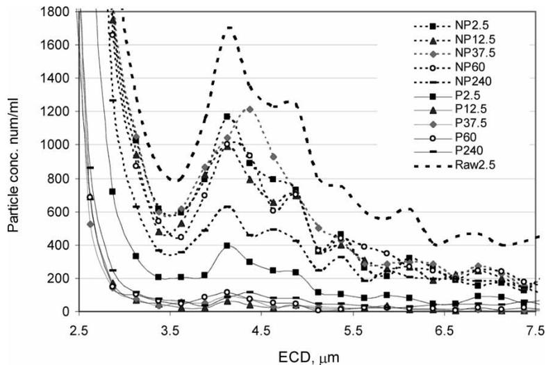
**Figure 1.** Particle size distribution (PSD) as a function of ECD filtered effluent with and without PAC. NP represents effluent of NPAC filter (dotted lines) while P represents effluent of PAC filter (full lines); Numbers in legend represent corrected time sample collected from filter effluent.
