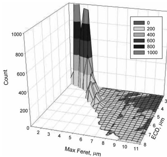
**Figure 7.** 3D plot of ECD as a function of feret max diameter for chlorine samples.
