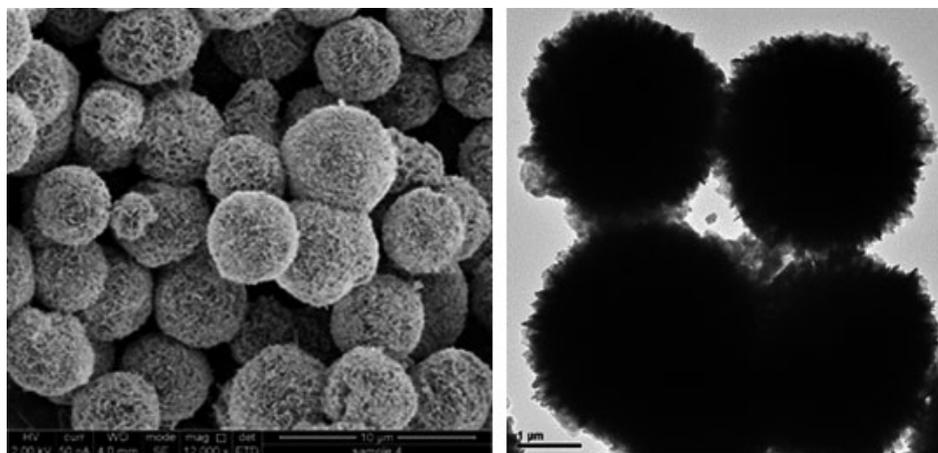
**Figure 2.** SEM (left) and TEM (right) micrographs of  $\text{BiOCl}_{0.875}\text{Br}_{0.125}$  photocatalyst.
