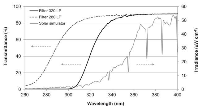
**Figure 3.** Solar simulator incident irradiation and transmittance for the selected filters as a function of wavelength.
