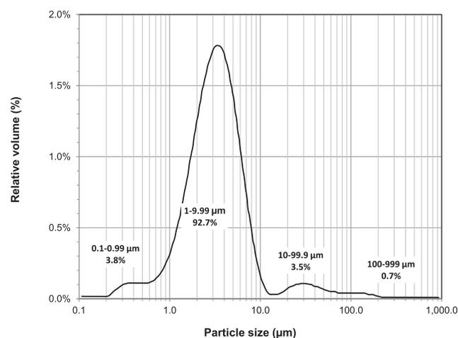
**Figure 1.** Particle size distribution of  $\text{BiOCl}_{0.875}\text{Br}_{0.125}$  photocatalyst.
