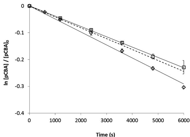
**Figure 2.** Degradation of pCBA in a 254 nm irradiated SRHA solution ( $15 \text{ mgC L}^{-1}$ ): ( $\Delta$ ) no added scavengers, ( $\square$ ) with 50 mM *t*-butanol, and (---) calculated direct photolysis.
