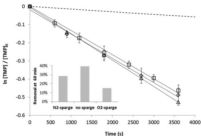
**Figure 4.** Degradation of TMP in a 254 nm irradiated SRHA solution (15  $\text{mgC L}^{-1}$ , pH 7): (◇) no added scavengers, (Δ) with 50 mM *t*-butanol, (□) with 1 mM FFA, and (---) calculated direct photolysis. Inset: influence of  $\text{N}_2$  and  $\text{O}_2$  sparging on % removal of TMP after 60 min irradiation.
