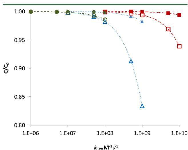
**Figure 5.** Expected removal of hypothetical organic contaminants during UV water treatment by photogenerated ( $\Delta$ )  $^3\text{DOM}^*$ , ( $\square$ )  $\text{HO}\bullet$ , and ( $\circ$ )  $^1\text{O}_2$ , as a function of the contaminants' rate constants for reaction with the different species. Filled and unfilled symbols correspond to UV doses at 254 nm of  $100 \text{ mJ cm}^{-2}$  and  $1000 \text{ mJ cm}^{-2}$ , respectively.
