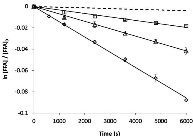
**Figure 1.** Degradation of FFA in a 254 nm irradiated SRHA solution ( $15 \text{ mgC L}^{-1}$ ): ( $\diamond$ ) no added scavengers, ( $\Delta$ ) with 50 mM *t*-butanol, ( $\square$ ) with 50 mM *t*-butanol and 1 mM  $\text{NaN}_3$ , and (---) calculated direct photolysis.
