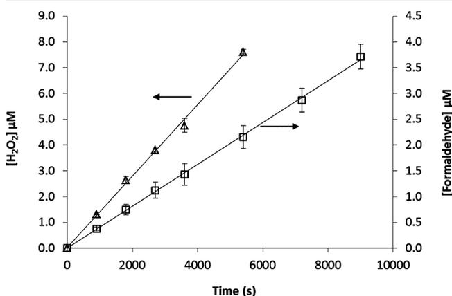
**Figure 3.** Concentration of (□) formaldehyde and (Δ)  $\text{H}_2\text{O}_2$  as a function of time in a 254 nm irradiated solution of SRHA (15  $\text{mgC L}^{-1}$ , pH 7). Experiments for formaldehyde conducted with 0.4 M methanol.
