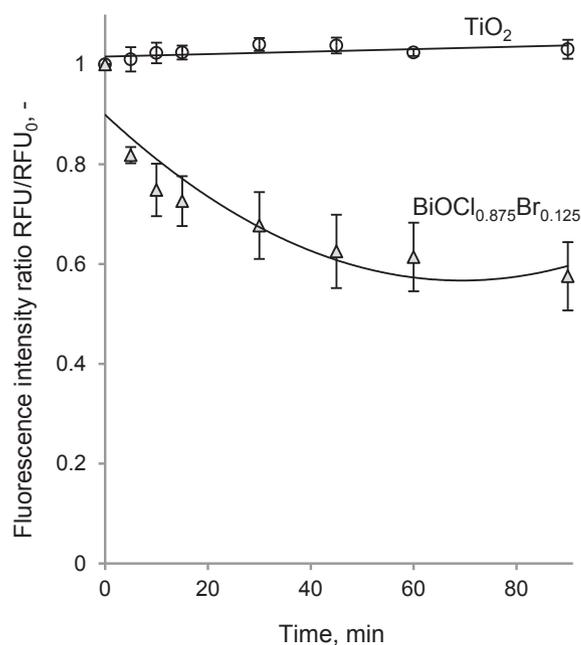
Fig. 6. Changes in fluorescence intensity of  $25 \text{ mg L}^{-1}$  free rhodamine B as a function of time due to adsorption to  $1 \text{ g L}^{-1}$   $\text{TiO}_2$  (circles) and  $1 \text{ g L}^{-1}$  bismuth ( $\text{BiOCl}_{0.875}\text{Br}_{0.125}$ ; triangles) in the dark.
