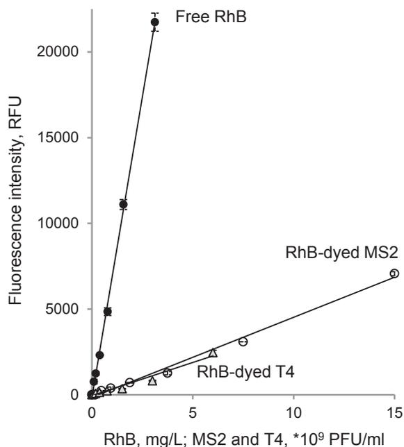
**Fig. 2.** Changes in fluorescence intensity as a function of concentration of 0–3.13 mg/l free rhodamine B (RhB) (full circles), 0–15 × 10<sup>9</sup> PFU ml<sup>-1</sup> RhB-dyed MS2 (empty circles) and 0–6 × 10<sup>9</sup> PFU ml<sup>-1</sup> RhB-dyed T4 (empty triangles).
