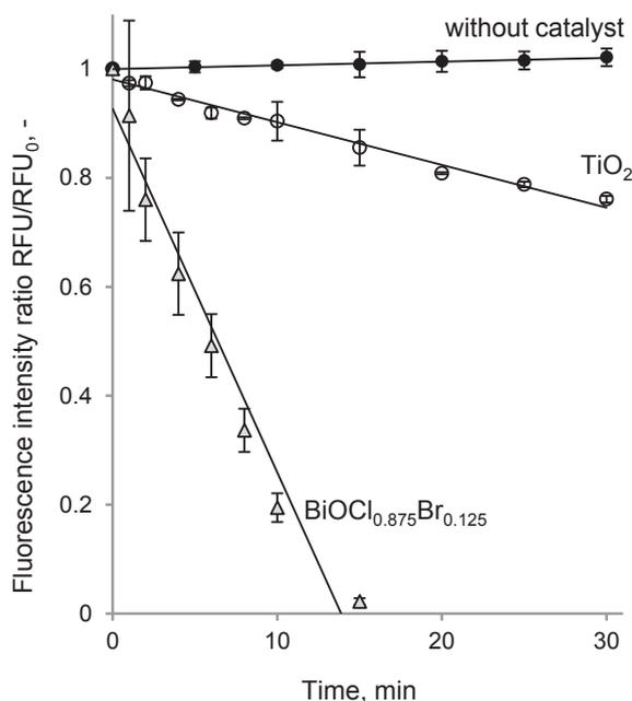
Fig. 5. Changes in fluorescence intensity of  $25 \text{ mg/l}$  free rhodamine B as a function of irradiation time using a 150-W xenon arc lamp solar simulator. Experiments were performed without catalyst (full circles) (pH 4.51), with addition of  $1 \text{ g L}^{-1} TiO_2$  (empty circles) (pH 4.70), and with addition of  $1 \text{ g L}^{-1}$  bismuth (empty triangles) (pH 4.88). Initial fluorescence intensity of RhB was 50,000 RFU (Synergy fluorimeter).
