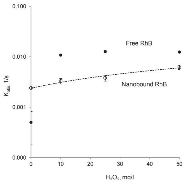
Fig. 4. Total degradation rate constant ( $k_{obs}$ ) as a function of  $H_2O_2$  concentration, for  $1 \text{ mg L}^{-1}$  free and  $4 \times 10^9 \text{ PFU ml}^{-1}$  nano-bound RhB by UV irradiation and AOP.
