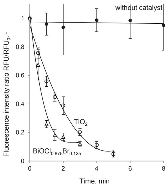
**Fig. 7.** Changes in fluorescence intensity of rhodamine B-dyed MS2 as a function of irradiation time using a 150-W xenon arc lamp solar simulator. Experiments were performed without catalyst (full circles), with addition of  $1 \text{ g L}^{-1}$   $\text{TiO}_2$  (empty circles), and with addition of  $1 \text{ g L}^{-1}$  bismuth ( $\text{BiOCl}_{0.875}\text{Br}_{0.125}$ ; empty triangles).
