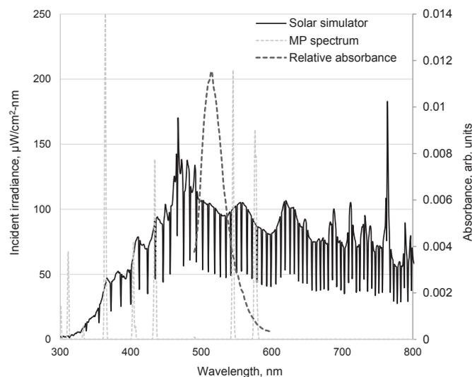
**Fig. 1.** Absorption spectrum of free rhodamine B and irradiation spectrum of medium-pressure (MP) UV and xenon arc lamp (solar simulator).
