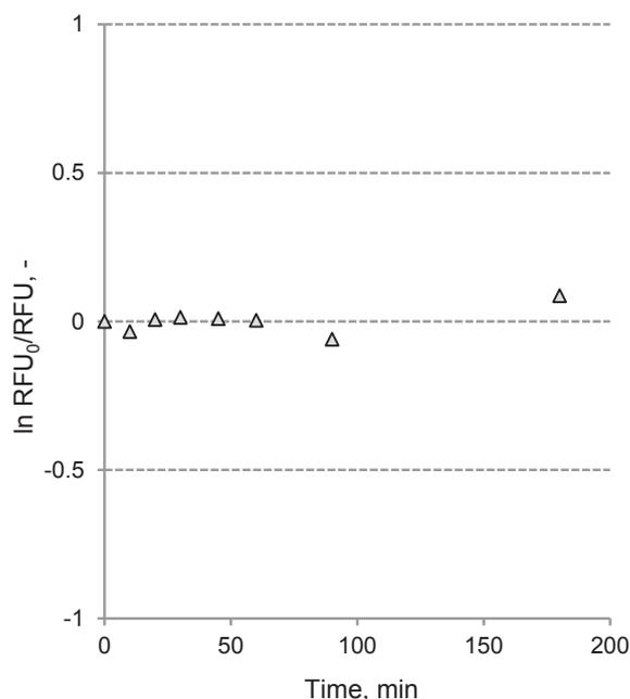
**Fig. 3.** Changes in fluorescence intensity of 1 mg L<sup>-1</sup> free rhodamine B (pH = 5.58) exposed to 100 mg L<sup>-1</sup> H<sub>2</sub>O<sub>2</sub> in the dark, as a function of time (pH = 5.58, with up to 100 mg L<sup>-1</sup> H<sub>2</sub>O<sub>2</sub>).
